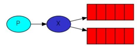
There are a few exchange types available: *DIRECT*, *TOPIC*, *HEADERS* and *FANOUT* (see *aio\_pika*. *ExchangeType*). We'll focus on the last one — the fanout. Let's create an exchange of that type, and call it *logs*:
