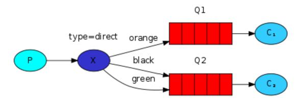
In this setup, we can see the *direct* exchange X with two queues bound to it. The first queue is bound with binding key *orange*, and the second has two bindings, one with binding key *black* and the other one with *green*.
