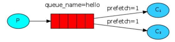
In order to defeat that we can use the basic.qos method with the *prefetch\_count=1* setting. This tells RabbitMQ not to give more than one message to a worker at a time. Or, in other words, don't dispatch a new message to a worker until it has processed and acknowledged the previous one. Instead, it will dispatch it to the next worker that is not still busy.
