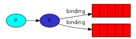
We've already created a fanout exchange and a queue. Now we need to tell the exchange to send messages to our queue. That relationship between exchange and a queue is called a binding.
