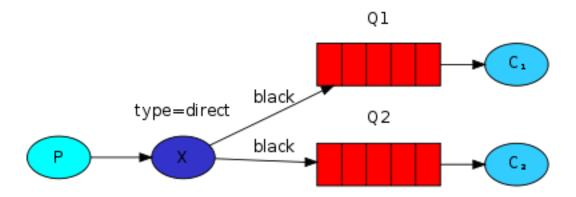
It is perfectly legal to bind multiple queues with the same binding key. In our example we could add a binding between X and QI with binding key black. In that case, the direct exchange will behave like fanout and will broadcast the message to all the matching queues. A message with routing key black will be delivered to both QI and Q2.
