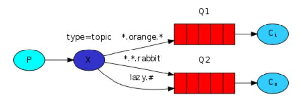
In this example, we're going to send messages which all describe animals. The messages will be sent with a routing key that consists of three words (two dots). The first word in the routing key will describe a celerity, second a colour and third a species: "<celerity>.<colour>.<species>".
