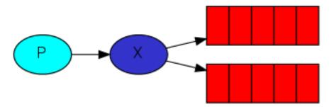
There are a few exchange types available: *DIRECT*, *TOPIC*, *HEADERS* and *FANOUT* (see <code>aio\_pika.ExchangeType</code>). We'll focus on the last one — the fanout. Let's create an exchange of that type, and call it *logs*:
