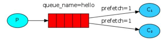
In order to defeat that we can use the basic.qos method with the *prefetch\_count=1* setting. This tells RabbitMQ not to give more than one message to a worker at a time. Or, in other words, don't dispatch a new message to a worker until it has processed and acknowledged the previous one. Instead, it will dispatch it to the next worker that is not still busy.
