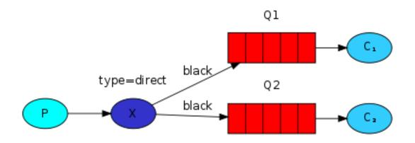
It is perfectly legal to bind multiple queues with the same binding key. In our example we could add a binding between X and Q1 with binding key *black*. In that case, the *direct* exchange will behave like fanout and will broadcast the message to all the matching queues. A message with routing key black will be delivered to both Q1 and Q2.
