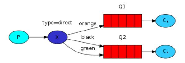
In this setup, we can see the *direct* exchange X with two queues bound to it. The first queue is bound with binding key *orange*, and the second has two bindings, one with binding key *black* and the other one with *green*.
