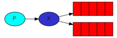
There are a few exchange types available: *DIRECT*, *TOPIC*, *HEADERS* and *FANOUT* (see <code>aio\_pika</code>. <code>ExchangeType</code>). We'll focus on the last one — the fanout. Let's create an exchange of that type, and call it <code>logs</code>:
