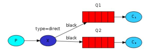
It is perfectly legal to bind multiple queues with the same binding key. In our example we could add a binding between X and Q1 with binding key black. In that case, the direct exchange will behave like fanout and will broadcast the message to all the matching queues. A message with routing key black will be delivered to both Q1 and Q2.
