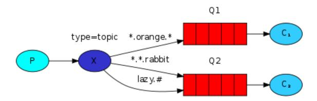
In this example, we're going to send messages which all describe animals. The messages will be sent with a routing key that consists of three words (two dots). The first word in the routing key will describe a celerity, second a colour and third a species: "<celerity>.<colour>.<species>"."
