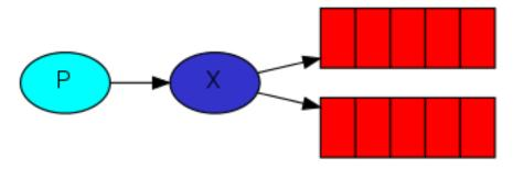
There are a few exchange types available: *DIRECT*, *TOPIC*, *HEADERS* and *FANOUT* (see <code>aio\_pika.ExchangeType</code>). We'll focus on the last one — the fanout. Let's create an exchange of that type, and call it *logs*:
